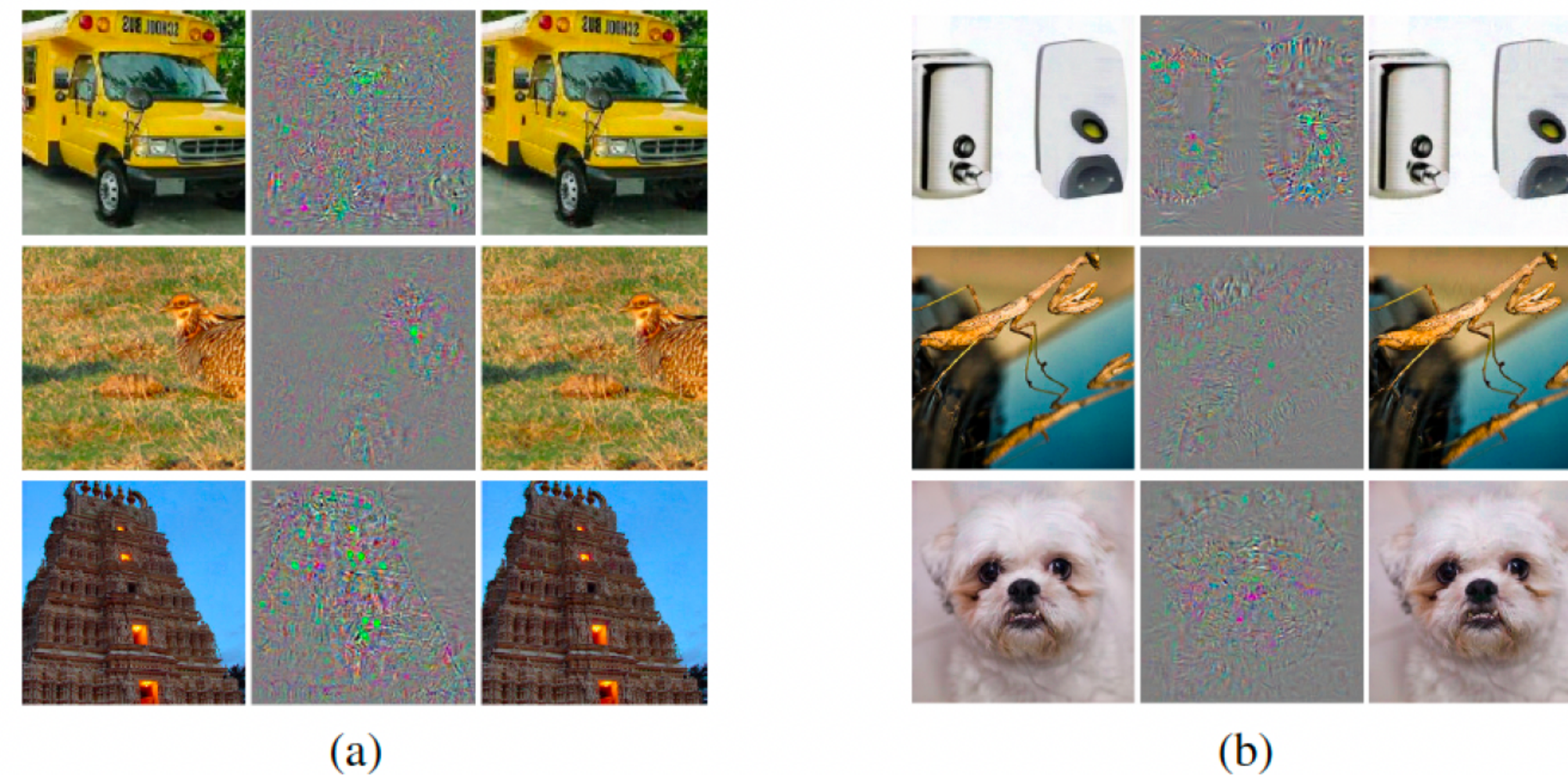
Figure 5: Adversarial examples generated for AlexNet [9].(Left) is a correctly predicted sample, (center) difference between correct image, and image predicted incorrectly magnified by 10x (values shifted by 128 and clamped), (right) adversarial example. All images in the right column are predicted to be an “ostrich, Struthio camelus ”. Average distortion based on 64 examples is 0.006508. Please refer to http://goo.gl/huaGPb for full resolution images. The examples are strictly randomly chosen. There is not any postselection involved.
